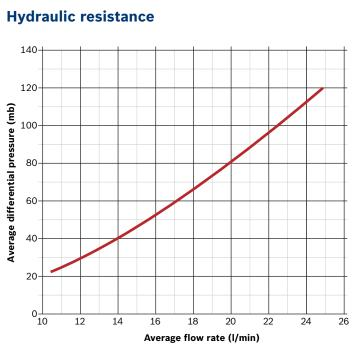
The above table provides water side resistance values to aid system design, pump head choice and pipework sizing.
