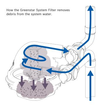
This cylindrical shape channels the water in an upwards spinning motion, assisting in the twin-action filtering process, whilst also providing a large capacity for captured system pollutants.
